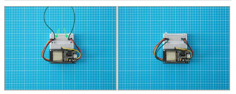
Connect the remaining leg (DOUT) of the lefthand LED to the leftmost leg (DIN) of the righthand
