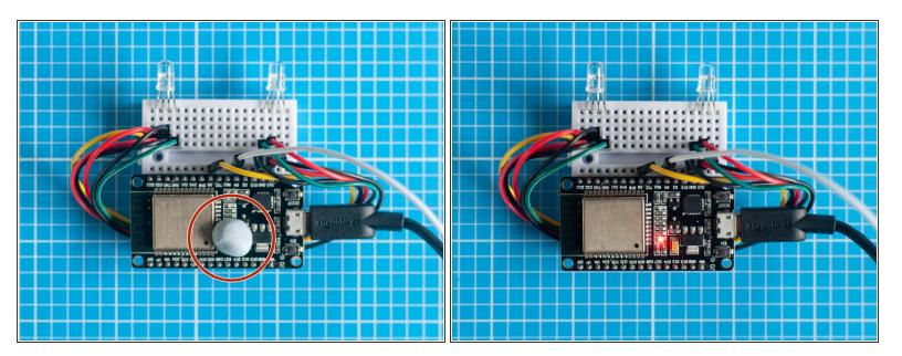
This step is optional, but the red power LED on the ESP32S board can seem quite bright in a darkened space and interfere with the main LED's. Covering this LED with a piece of Blu Tack or tape will eliminate the issue.
