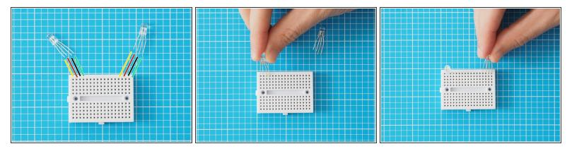
Place LEDs in breadboard as pictured. Make sure the orientation of the LEDs are the same (short legs to the left of the breadboard)
