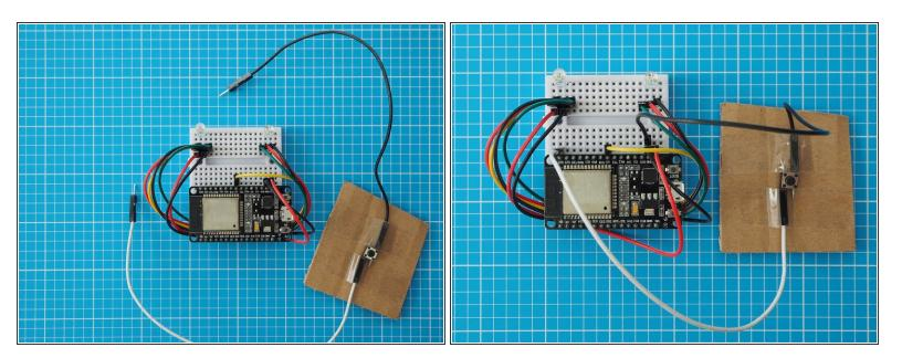
An external Button can be used instead of capacitive touch by adding a switch between pin D23 and GND on the ESP32.
