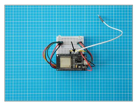
Add the final jumper wire in line with ESP32 pin D4.
