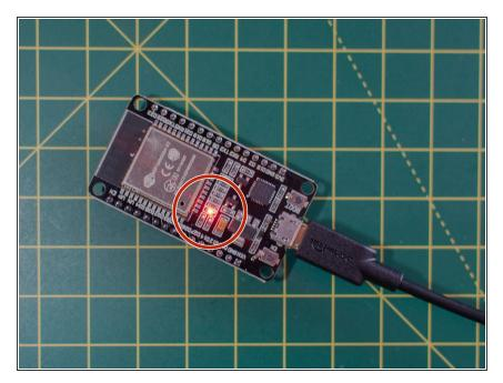
Plug your ESP32S board into your computer with the USB cable. You should see a red light on the board, which means it is powered up.
