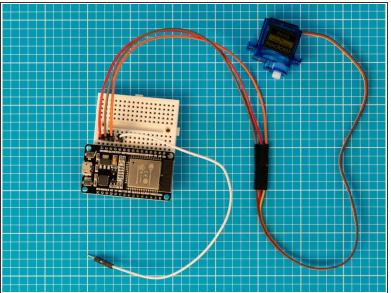
Add the final jumper wire in line with ESP32S pin D14.
