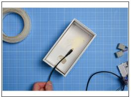
Using the mark you made in the previous step, mark and cut a slot in the inner sleeve large enough for the USB lead to pass through.
