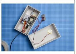
Attach a small piece of double-sided tape to the rear (the brass disc) of the piezo sensor and mount on the inside of the outer sleeve or lid of the box.
