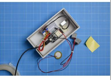
In most cases, the breadboard will already have a self-adhesive pad on the rear (use double-sided tape if not). Peel away the protective layer and stick the breadboard inside the box.
