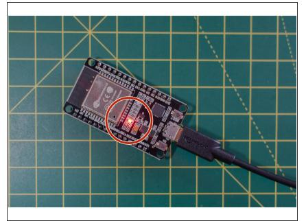
Plug your ESP32S board into your computer with the USB cable. You should see a red light on the board, which means it is powered up.
